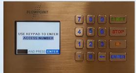
1. Using the Keypad, type in the Access Code and then press <mark>ENTER</mark>.
