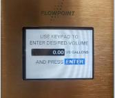
4. Enter in the desired volume of Water (Gallons) and press <mark>ENTER</mark>.
