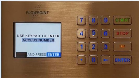
1. Using the Keypad, type in the Access Code and then press **ENTER**.
