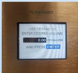
4. Enter in the desired volume of Water (Gallons) and press **ENTER**.
